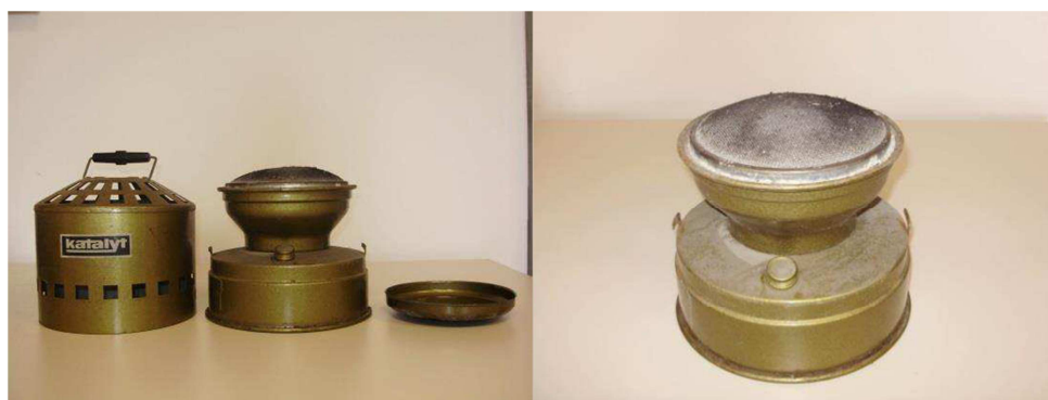
Fig. 3: Catalytic heaters containing asbestos
